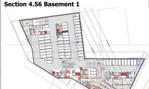
7. The basement levels have been split with a level difference introduced to each level to allow for the additional headroom requirements for the waste and service vehicles of 4.5m at Basement 1 level
